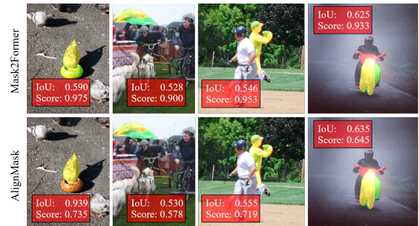
Fig. 1. Illustration of segmentation results (mask IoU with Ground-truth and classification scores) predicted by Mask2Former [8] (top row) and the proposed AlignMask (bottom row). Ground-truth is indicated by red mask, prediction is green mask, and there overlap is yellow mask. Classification scores predicted by AlignMask better reflect the segmentation quality of mask.
